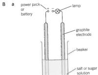
make up separate solutions of each substance in small beakers; place the two electrodes in one of the beakers, and switch on the current; if the bulb lights, the substance is sodium chloride; if the bulb does not light, the substance is sugar; repeat the experiment with the other solution
